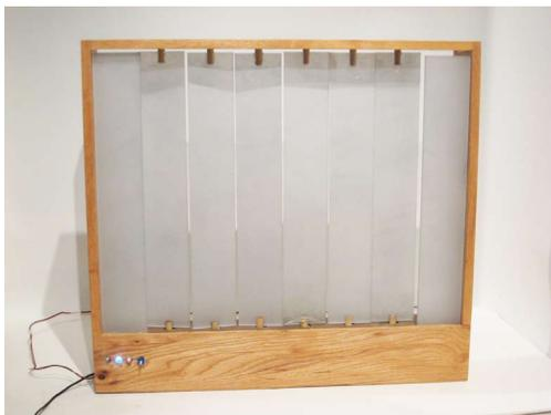
**Figure 10: Fully Closed Louvers**
